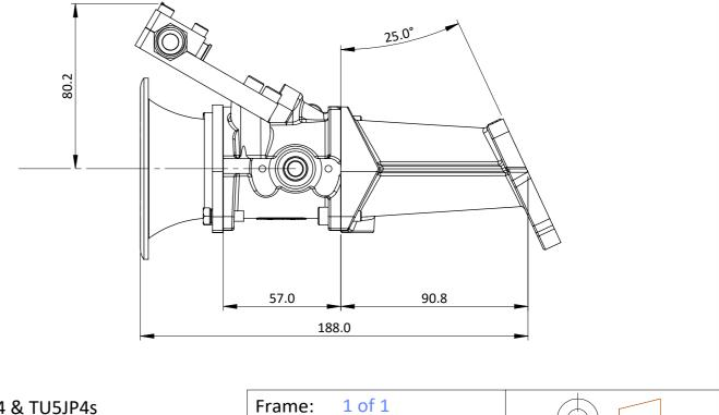
The Jenvey Dynamics tapered CKPG04 kit promises enhanced performance and better throttle control for the TU5JP4 & TU5JP4s engine as found in the VTS, VTR & GT models. This kit contains, an inlet manifold, four ST45 tapered throttle bodies (42mm butterfly), fuel rail, fuel rail mounts and 40mm long airhorns.
