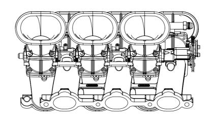
A KIT FOR THE NISSAN VQ SERIES ENGINE WHICH INCLUDES A PAIR OF MANIFOLDS, SIX 51mm SF51 TAPERED BODIES, LINKAGE, FUEL RAILS WITH DASH 6 ENDS AND SIX AHT51X110X40 CURVED OVAL ENRTY AIRHORNS. (DOES NOT INCLUDE INJECTORS) THIS SPECIAL KIT IS DESIGNED TO FIT UNDER THE 350Z BONNET. THE ENGINE IS USED BY INFINITI IN SEVERAL MODELS IN THE US AND THE 350Z IN THE UK AS WELL AS CERTAIN RENAULTS. MADE TO ORDER.
