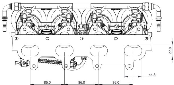
A KIT FOR RIGHT HAND DRIVE 1.6L MX5'S, WHICH INCLUDES A DCOE INLET MANIFOLD, 90MM LONG TH THROTTLE BODIES, FUEL RAIL AND AIRHORNS.
