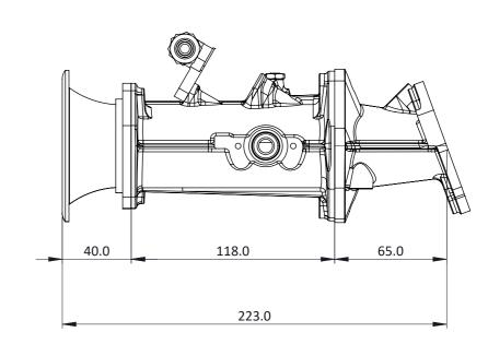
A TWIN THROTTLE BODY KIT FOR THE MK1 & MK2 MAZDA MX5 1.8L NA ENGINE.
