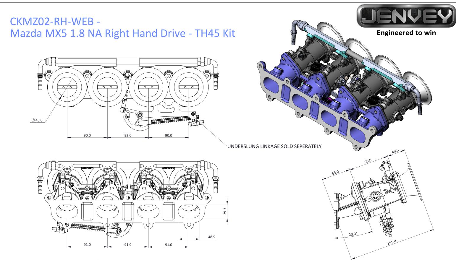
A KIT FOR RIGHT HAND DRIVE NA 1.8L MX5'S, WHICH INCLUDES A DCOE INLET MANIFOLD, 90MM LONG TH THROTTLE BODIES, FUEL RAIL AND AIRHORNS.
