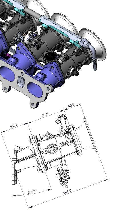
A KIT FOR RIGHT HAND DRIVE NB 1.8L MX5'S, WHICH INCLUDES A DCOE INLET MANIFOLD, 90MM LONG TH THROTTLE BODIES, FUEL RAIL AND AIRHORNS.
