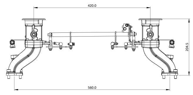
Flanges for Jenvey single (SF, SFS) throttle bodies. Ø48mm bodies with sufficient material in manifold to allow matching to ported cyclinder heads.
