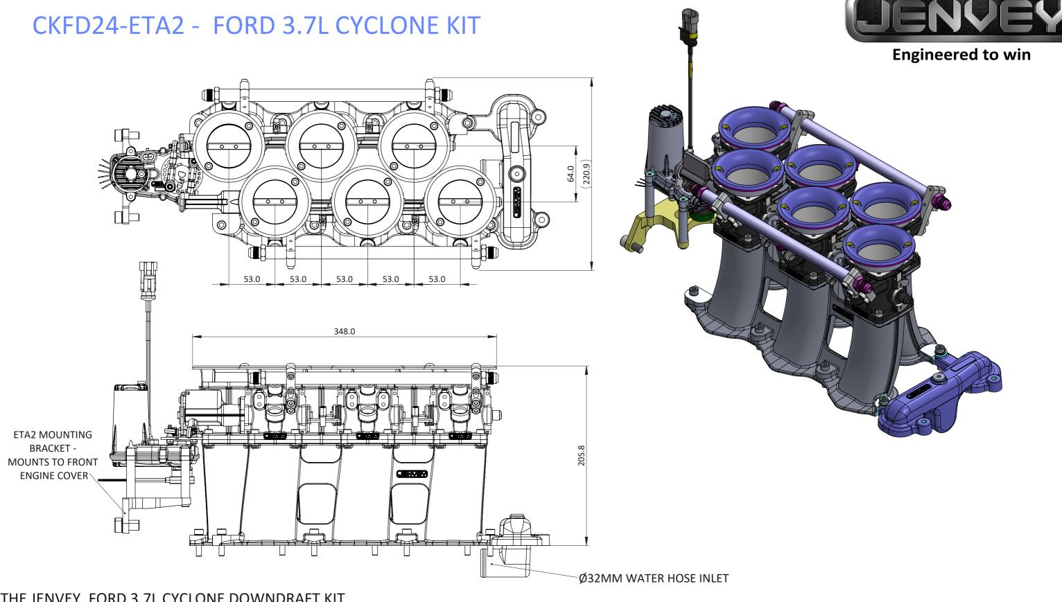
THE JENVEY, FORD 3.7L CYCLONE DOWNDRAFT KIT INCLUDES MANIFOLDS, Ø51MM SF THROTTLE BODIES, 19MM AIRHORNS, FUEL RAILS + MOUNTS, \*WATER MANIFOLD, JENVEY ETA2, MOUNTING BRACKET & LINKAGE, & TP3 THROTTLE POSITION SENSOR.
