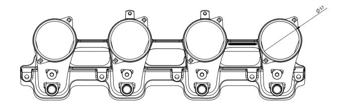
FLANGES FOR JENVEY SSD THROTTLE BODIES. SUFFICIENT METAL TO ALLOW PORT MACHINING. 'O' RING SEAL ONTO CYLINDER HEAD. INCLUDES INJECTOR POCKETS AND EXTRA UNDRILLED BOSSES FOR IDLE AIR / VACUUM TAKE OFF
